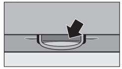
■ The lower part of the inner door has a drip tray. Clean the drip tray.
